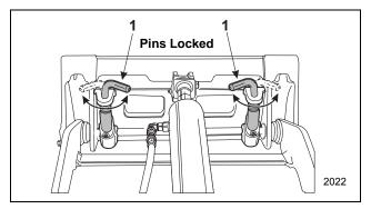
Figure 3–23 Attachment Locks in Locked Position
